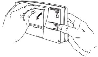
3. Slide the catch to rest the kickstand in the appropriate angle.
