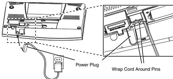
3. Insert the power adapter plug into the console power jack, then plug the other end of the adapter into an appropriate power outlet.
