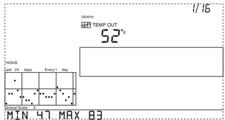
By pressing the down arrow again, the graph shifts to show the highs of the last 24 months. As before, use the right and left arrows to move between months. Press HI/LOW to shift between the highs and lows.
